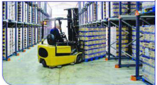
Drive in Racking System
